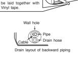
Connecting cords, pipe and drain hose must
